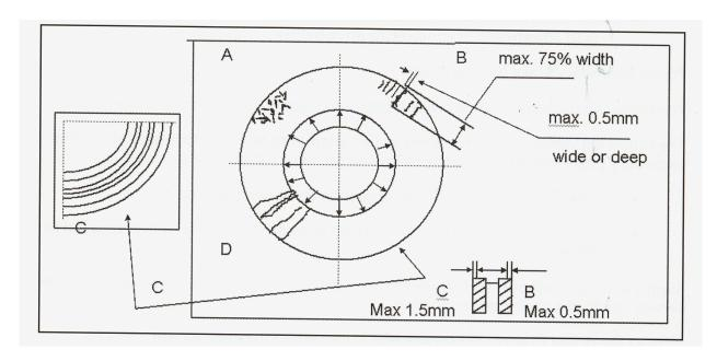
**Reservoirs** (The term reservoir includes accumulators and other types of vacuum & pressure vessels).
