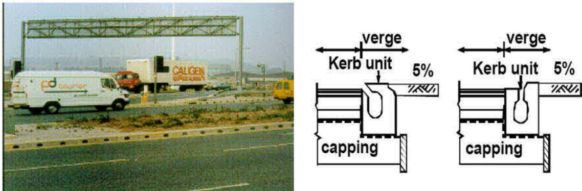
Figure 3.5 - Typical combined kerb and drainage unit
