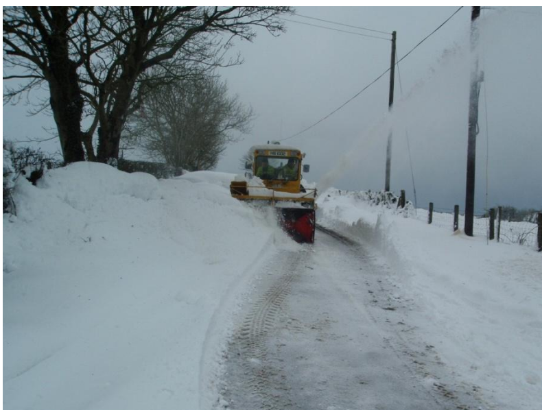
A Snow Blower in operation within Southern Division.
