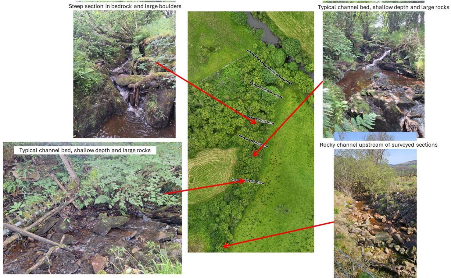
Figure 5-3: Lower reach of Curraghinalt Burn showing cross-section locations and key geomorphological features
