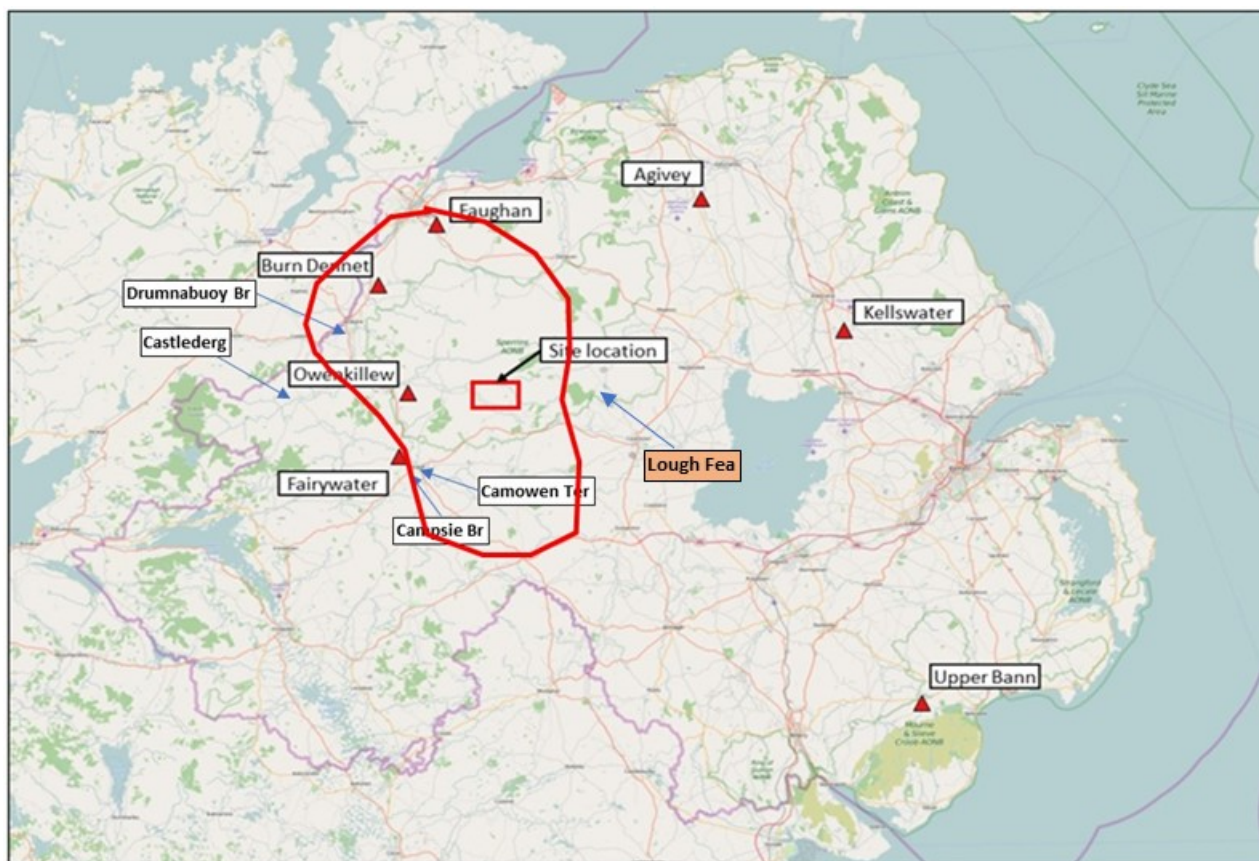
Figure A1: Location of Rivers Agency gauging stations used in analysis. Red boundary shows area where the 2017 event appears to have had the largest impact on the AMAX time series
