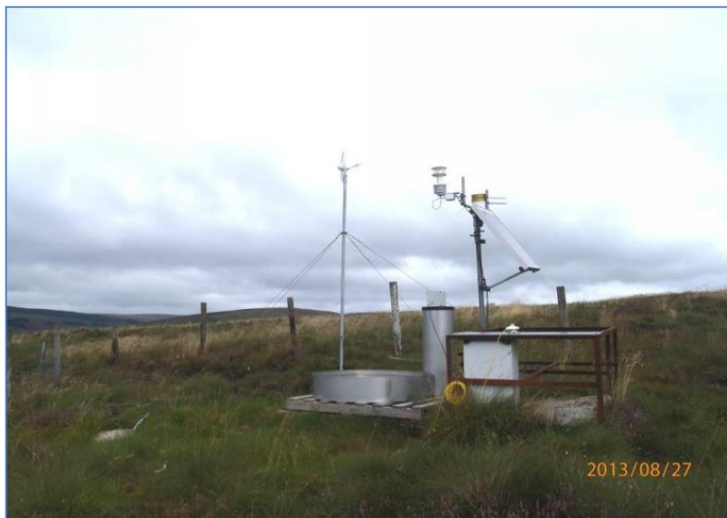
Photo 2: Curraghinalt Meteorological Station with evaporation pan, pyranometer and wind vane (SLR, 2013)
